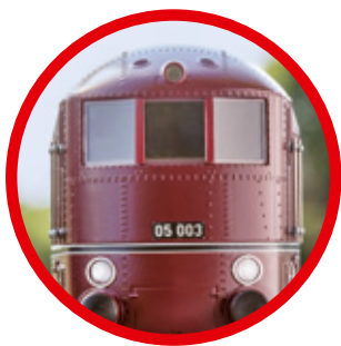
Innovative front engineer's cab with large windows, headlights and 'train approaching' light.
