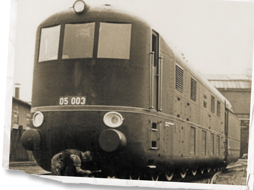
Looking ahead: the aerodynamic engineer's cab of 05 003 was to influence the 'face' of future express locos. On the front at the top, the 'train approaching' light.
