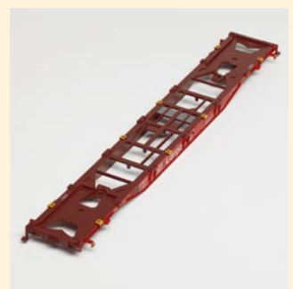
Stage 4: In the paint shop, the car floor is undercoated and top-coated, and painted as required for variants. Lettering takes 48 separate working steps.
