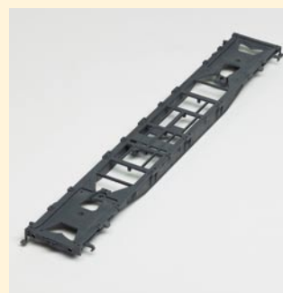
Stage 3: In the galvanic bath the surface is treated to a protective coating of phosphate solution against corrosion and to improve color adhesion.
