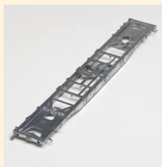
Stage 2: In the casting processing, the part is deburred by brushing and mechanically. CNC-processing is sometimes also used for drilling for attachments.
