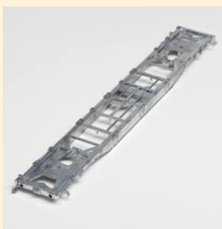
Stage 1: the die-cast blank comes out of the mold, rigid but 250°C hot and when cooled down, it is immediately subjected to searching optical inspection.
