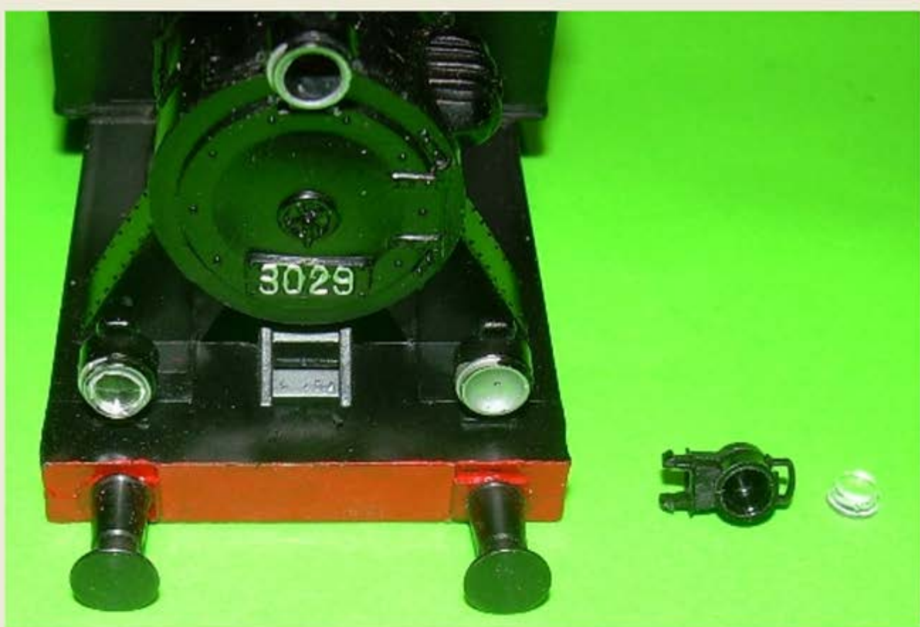
Install lanterns at the front. Upper lantern drilled out, lower left with lens inserted.
