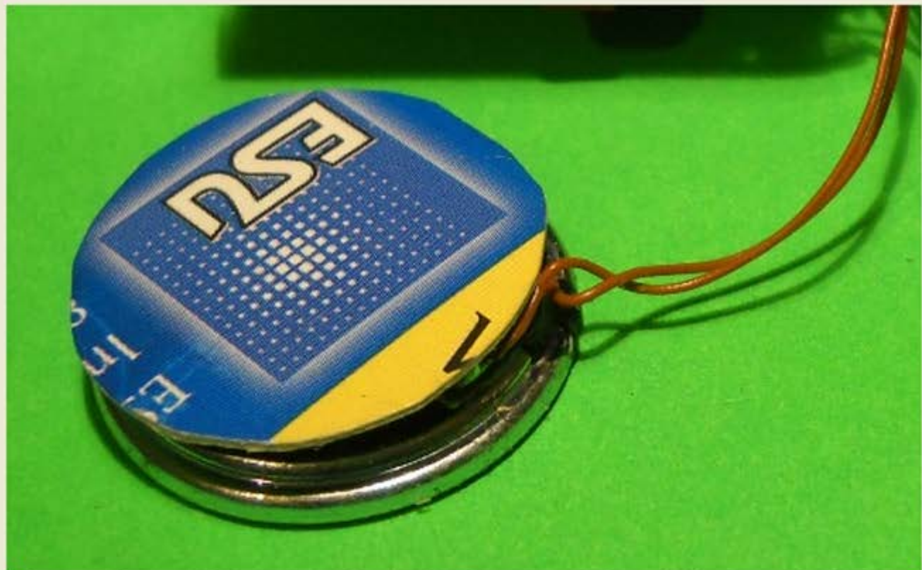
The speaker get its own very flat baffle, just a card board glued on the back, ...
