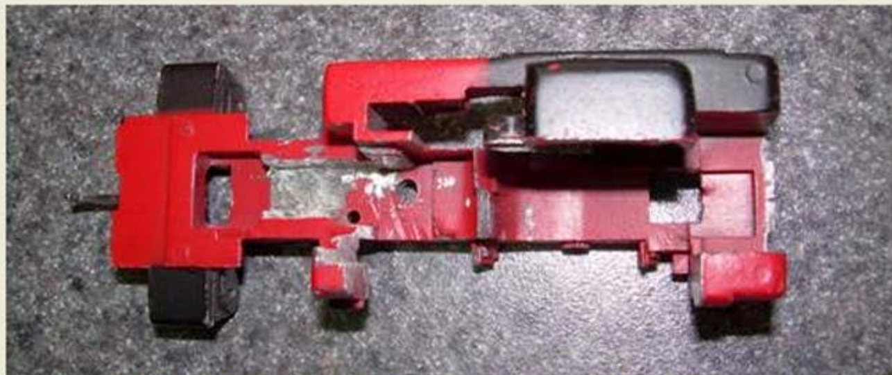
More milling in the front of the frame for the decoder and one speaker.
