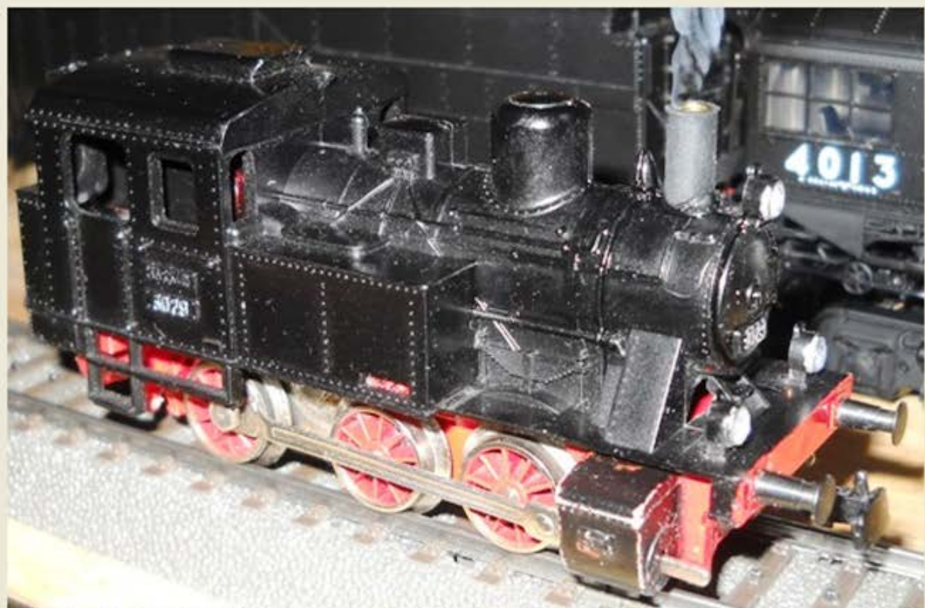
Märklin 3029 with 16 functions installed, includes smoke and front and rear lights.
