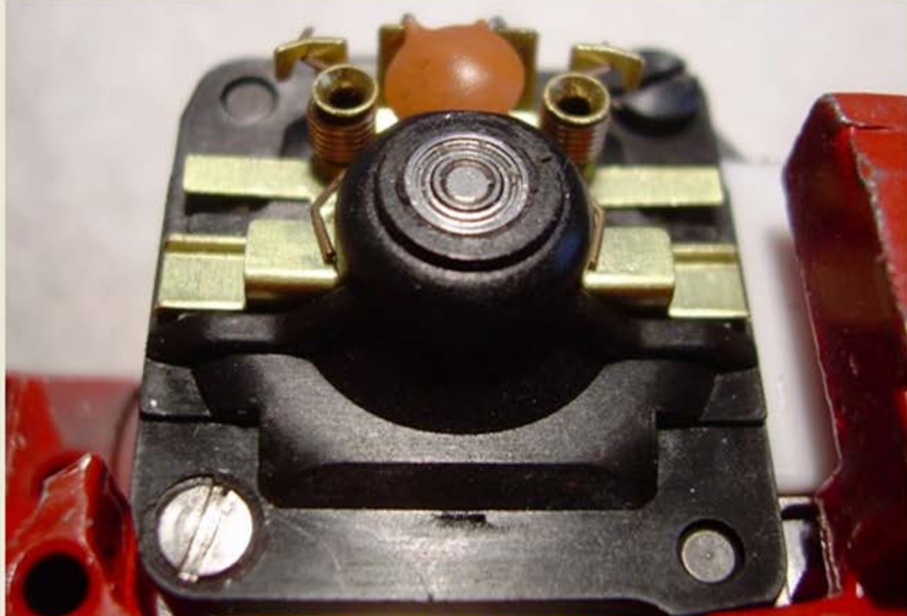
Ball bearing installed in the brush holder plate
