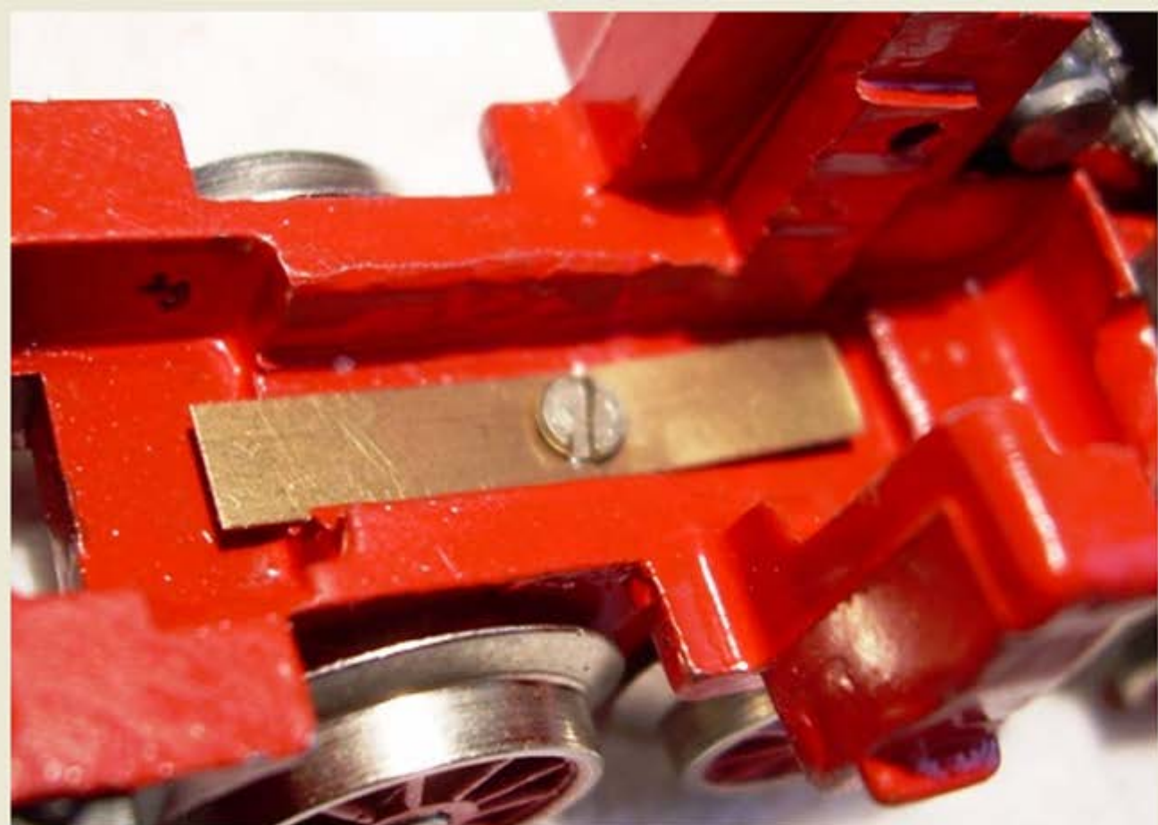
Underneath the brass bracket are two contact springs on both front axles.
