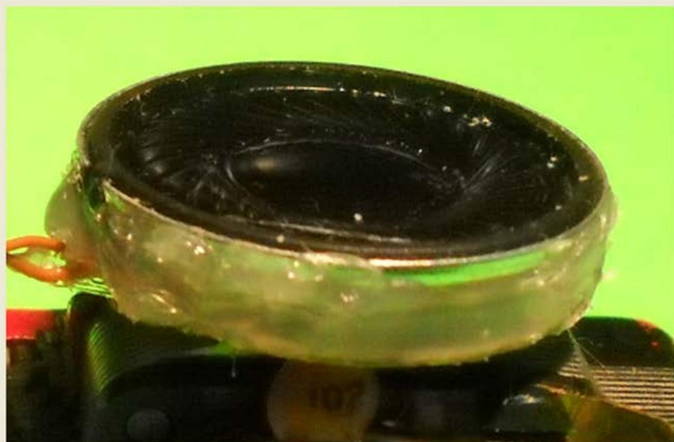
... completely sealed with hot glue, and mounted in the cabin under the roof.
