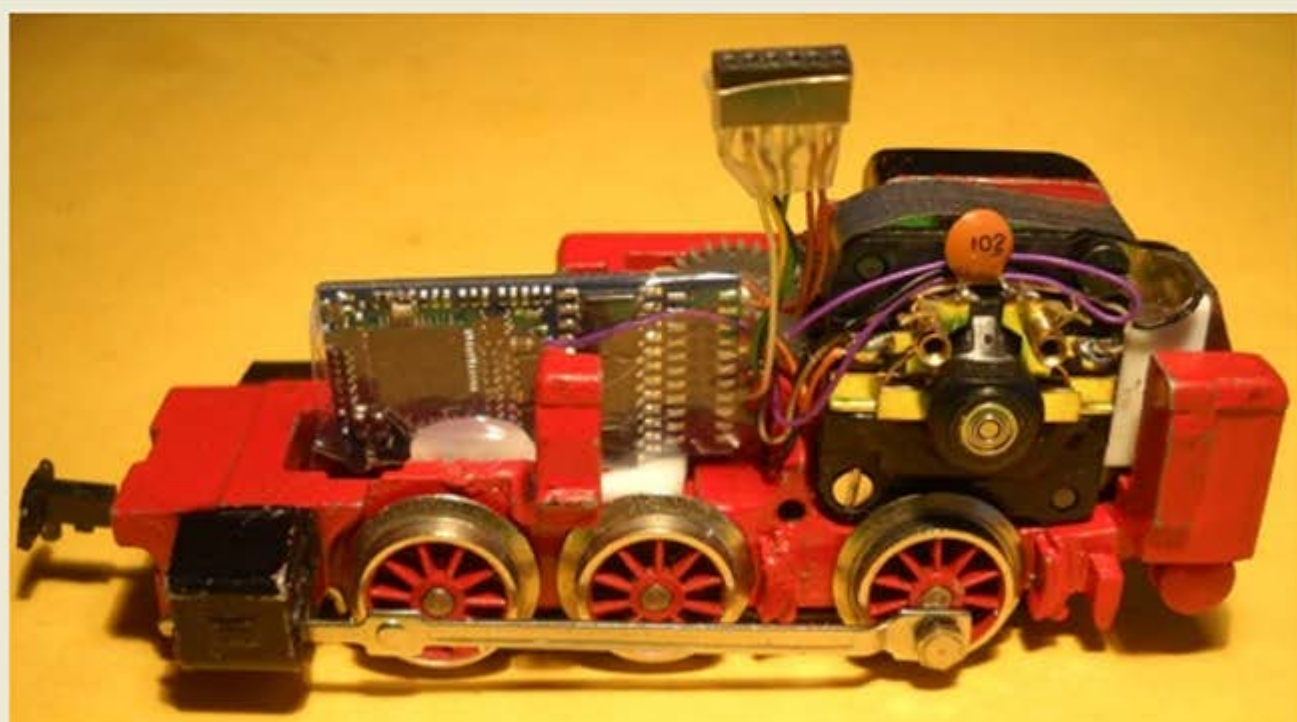
ESU LokSound M4 (mfx®) decoder and NEM 651 6-pin connector installed.
